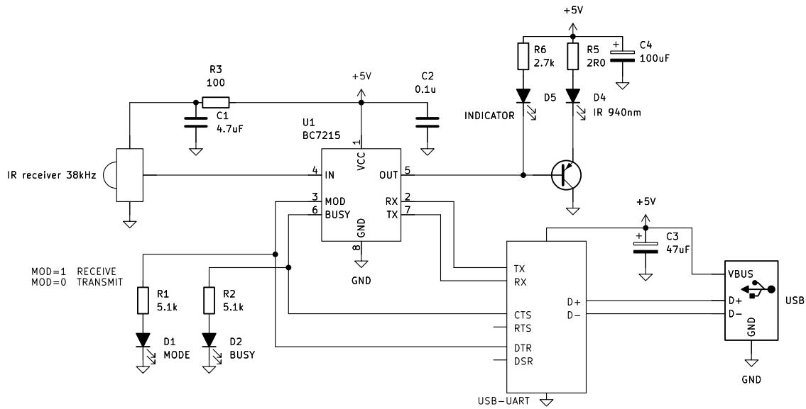
(When connected to a computer, please ensure that your device driver supports the hardware flow control of the USB-UART chip. Otherwise, the BC7215's UART buffer might overflow, causing the failure of long frame sending.)
