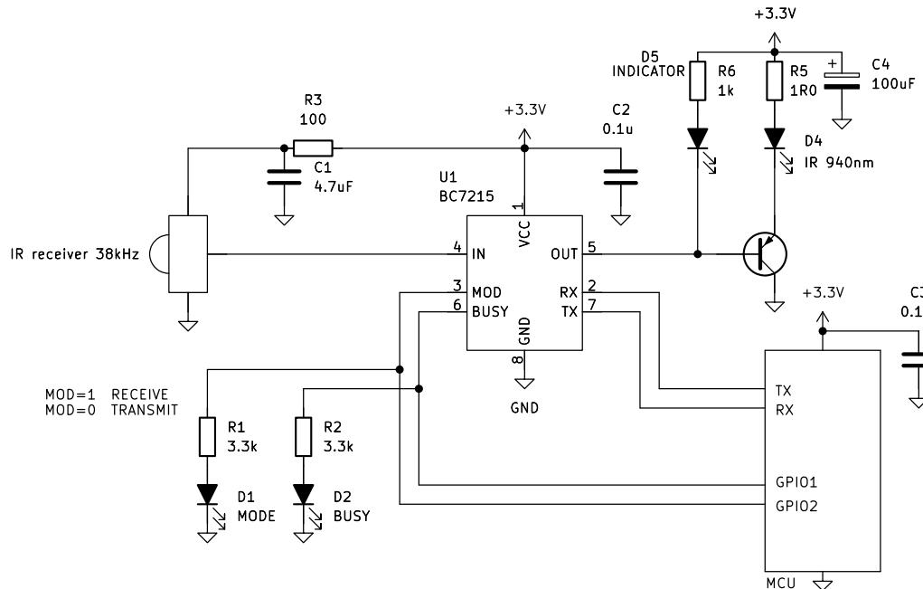
Infrared LEDs generally require a relatively high peak current to achieve longer transmission range. Many infrared LEDs can withstand peak currents of up to 1A. During transmission, the average working current of an infrared LED (with carrier) can exceed 200mA. This significant current demand should be carefully accommodated in the design of the power supply.
